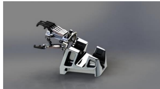
Figure 1. Hand exoskeleton and forearm support
