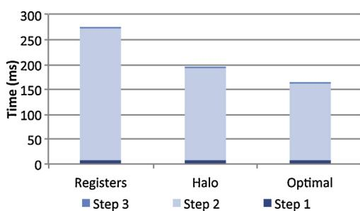
**Fig. 5 – Time comparison for GPU implementations of Cross-ApEn for steps described in Section 2.1.** The times showed correspond to the computation over 50 independent trials of size 8192. Step 2 performance varies depending on Registers, Halo and Optimal implementations described in Section 3.2. The latter is  $43\%$  faster than the first.
