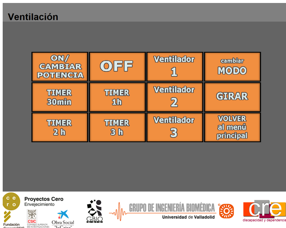
Figure 24. Snapshot of the Fan submenu. The user can manage different functions commonly present in a Fan remote control as well as go back to the Main menu.
