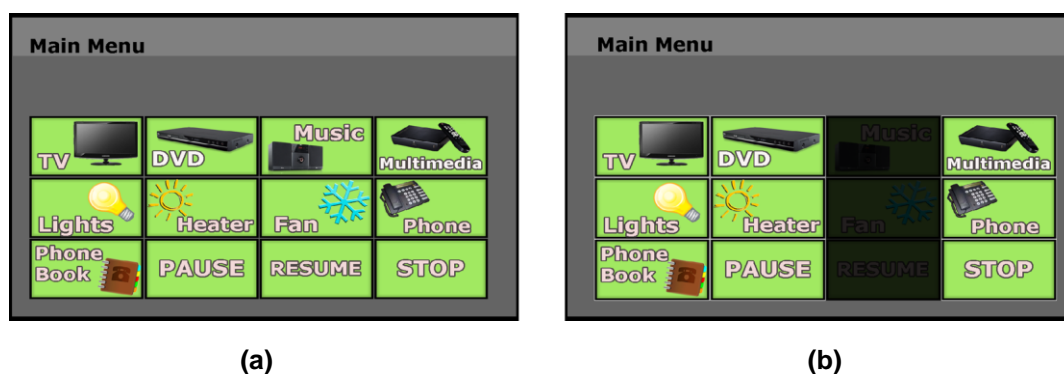
Figure 17. Snapshot of the assistive tool: (a) Main menu: it shows a 3x4 matrix consisted of images depicting all available devices: TV, DVD player, Hi-Fi system, multimedia drive, lights, heater, fan, and phone. (b) Main menu while the third column is dimmed.
